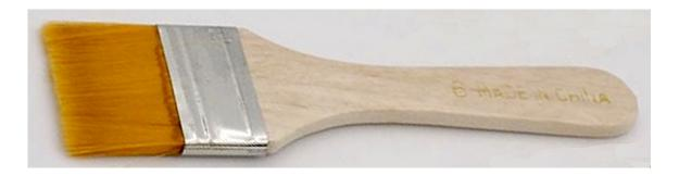
It is best to use the thin wide brushes made for varnishing. These have very fine points on the bristles so brush marks are much reduced. Avoid going back over the coat, as after a minute or two this will show brush marks anyway. Brushes are washed in water. I found it fine to leave the brush in water between coats. All that is needed is to wipe the brush dryish on a cloth or paper towel before using it again. I bought a set of three (25, 37 and 50 mm) on Ebay for £3.85.
